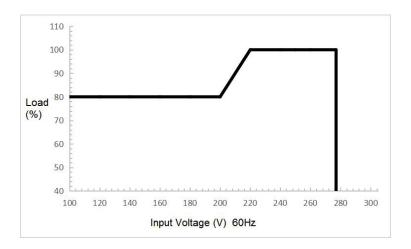
Remark: The output derating happens when the input voltage is low.
