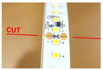
2) If a wiring tail is not present on the strip, you must solder one on now before continuing. A soldering iron 30-50W should be used. Any less or more\* will make the process overly difficult. The goal is to have about 2mm of cable tinned with solder.
