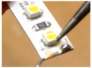
Attach the red wire to the (+) pad and the black wire to the (-) pad. Very little extra solder should be required to fuse the two pre-tinned items together. Once soldered the joints Check the reverse side too - that there is no excess solder should be bright and glossy. If not, more heat is required: showing here:
