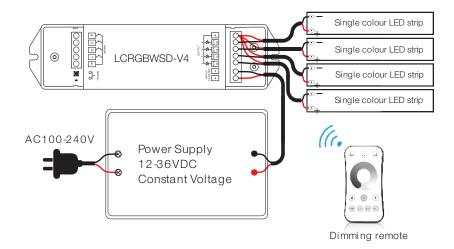
· LCRGBWSD-V4 with four push key for 4 channel single colour
