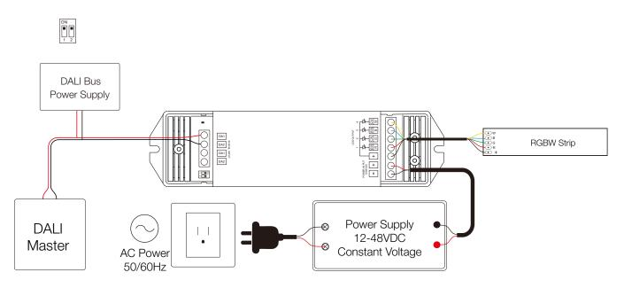
This product is designed with 1 DALI address input and 4 channel outputs, DALI address is assigned by the DALI Master controller automatically.
